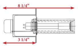
Oxidizing unit box size is 4 1/8" high x 4 1/8" wide. Lamp socket size is 3.5" x 2.75" x 1.625" Power box size is 6" x 5.75" x 1.5"
