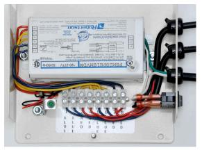
For dual lamp operation connect matching colored lamp wires to terminals. LampA Blue 1 - 2 Red 3 - 4 Lamp B Blue 5 - 6 Red 7 - 8
